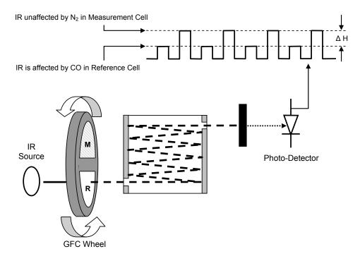
Figure 13-3: Measurement Fundamentals with GFC Wheel
